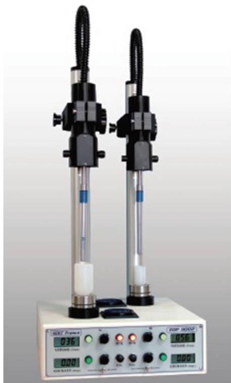
Fig. 1 (color online) The electrodeposition instrument of EDP 9002
