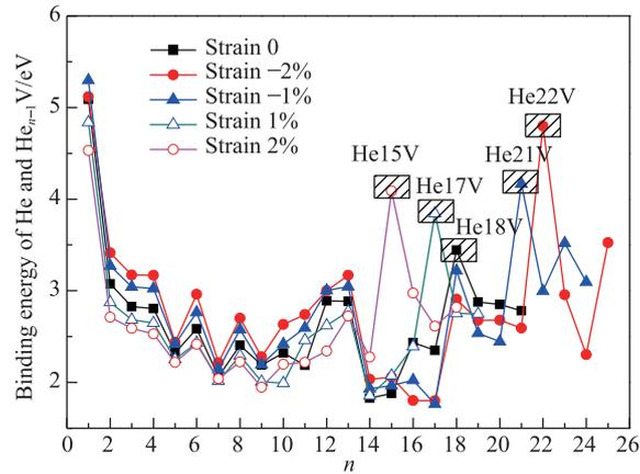
Fig. 1 (color online) The binding energies of He and  $\text{He}_{n-1}\text{V}$  under different strains. The inserted boxes corresponds to the first SIA emission.
