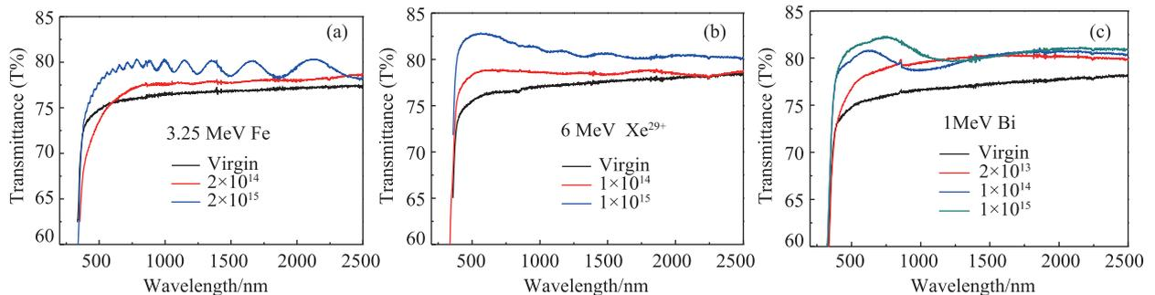
Fig. 1 (color online) The transmission spectra of LiTaO<sub>3</sub> implanted with Fe, Xe, Bi ions respectively at different fluences.
