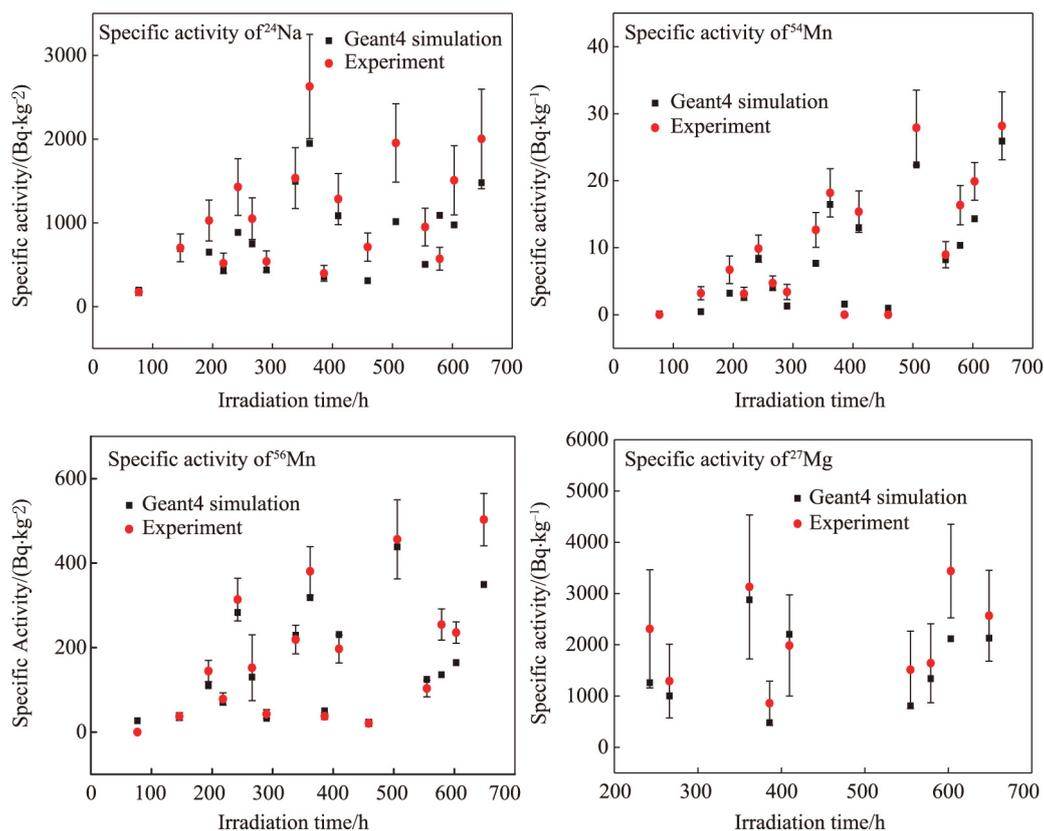
Fig. 1 (color online) The specific activities of induced-nuclides  $^{24}\text{Na}$ ,  $^{54}\text{Mn}$ ,  $^{56}\text{Mn}$  and  $^{27}\text{Mg}$  in pebble samples.
