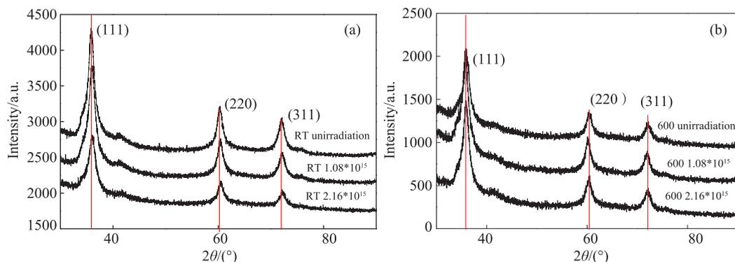
Fig. 2 (color online) XRD spectra of irradiated and non-irradiated SiC fibers. (a) at RT (b) at 600 °C.
