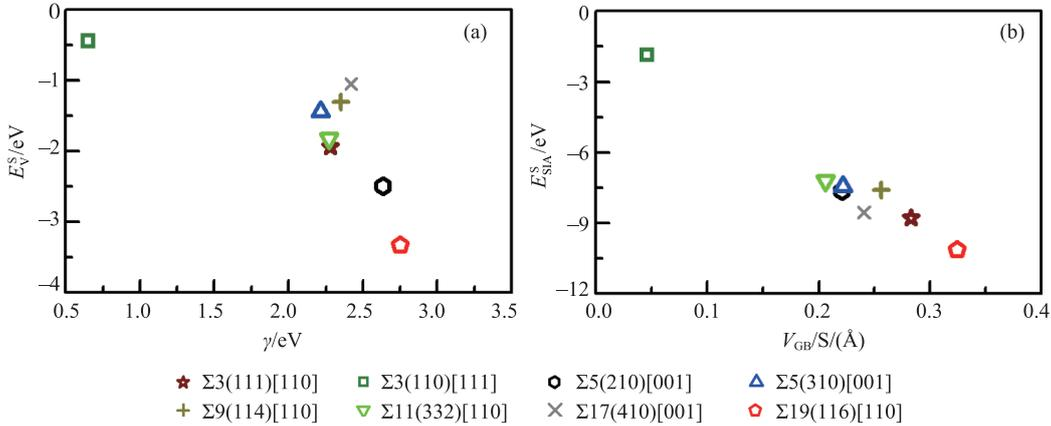
Fig. 1 (color online) (a) Dependence of the segregation energy  $E_V^S$  of V on GB energy  $\gamma$  and (b) dependence of the segregation energy  $E_{SIA}^S$  of SIA on excess volume  $V_{GB}/S$  of GB.
