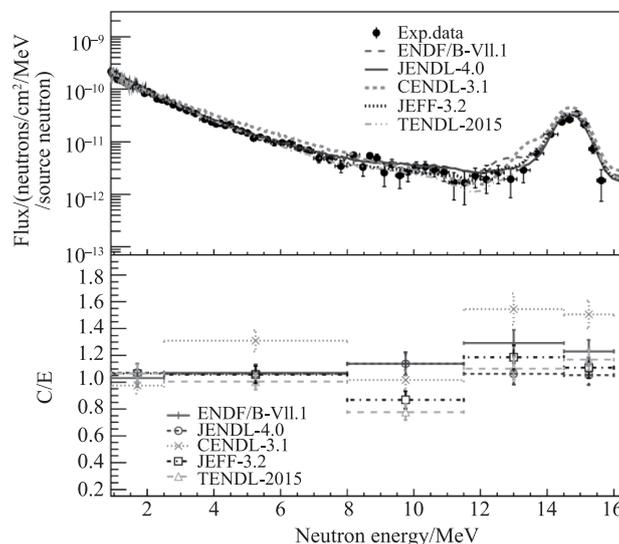
Fig. 1 Comparison of measured and calculated leakage neutron energy spectra for 14.8 MeV neutron on a  $^{238}\text{U}$  sample (10 cm $\times$ 10 cm $\times$ 2 cm).
