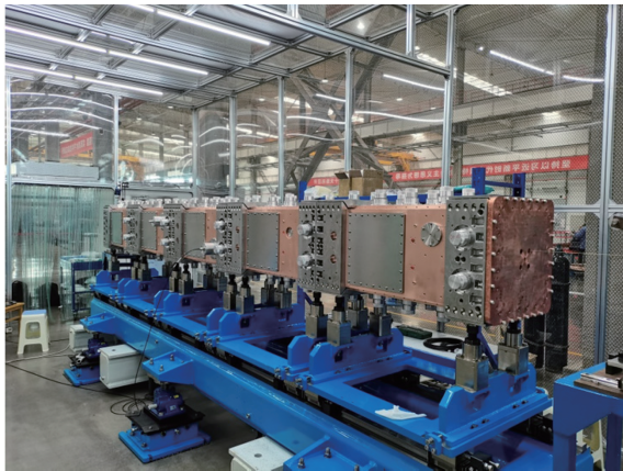
Fig. 1 (color online) The CiADS RFQ cavity Field under tuning and RF measurements.
