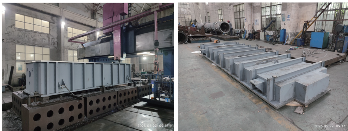
Fig. 1 (color online) Vacuum vessel manufacturing for CiADS cryomodule prototype.
