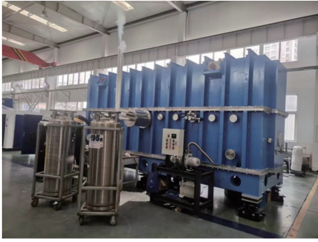
Fig. 2 (color online) Liquid nitrogen testing for HIAF cryomodule prototype.
