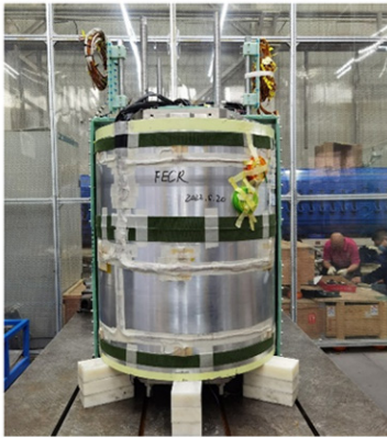
Fig. 2 (color online) The picture of the assembly for FEER full-length cold mass.
