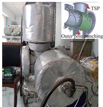
Fig. 2 (color online) Experimental setup with a 720-holes BPM.
