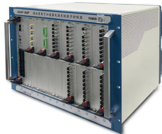
Fig. 1 (color online) The series of digital controller SZF-3. The left panel is the SZF-3-F1D1. The right panel is the SZF-3-F2E.
