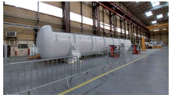
Fig. 2 (color online) Picture of the cold box bottom half.
