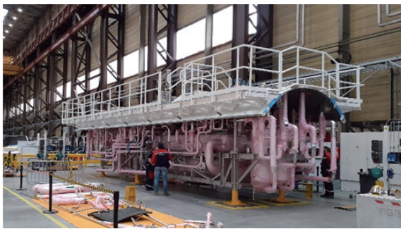
Fig. 1 (color online) Picture of the cold box top half.
