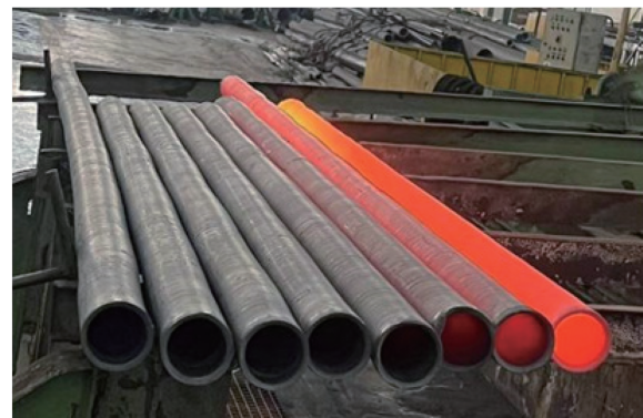
Fig. 2 (color online) Billet tubes of the SIMP-exchanger after hot piercing.
