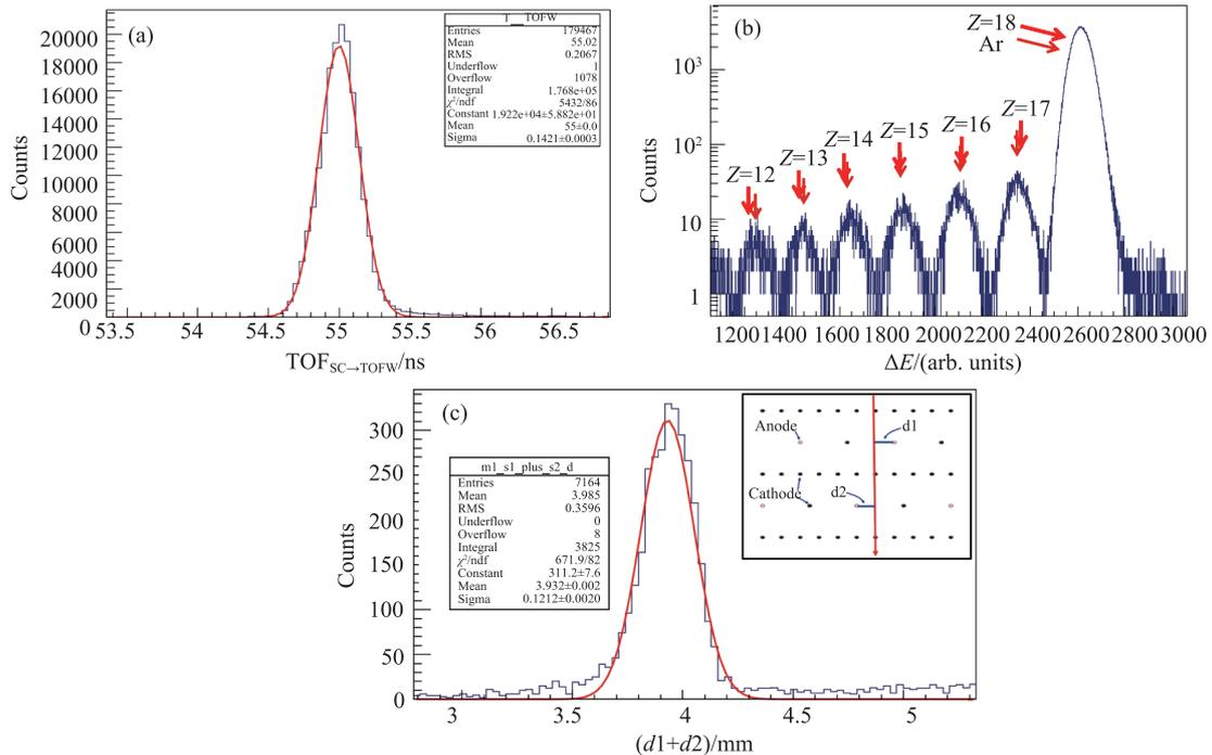
Fig. 2 (color online) Results of the resolution of (a) time of flight, (b) charge number and (c) position of ETF detectors.
