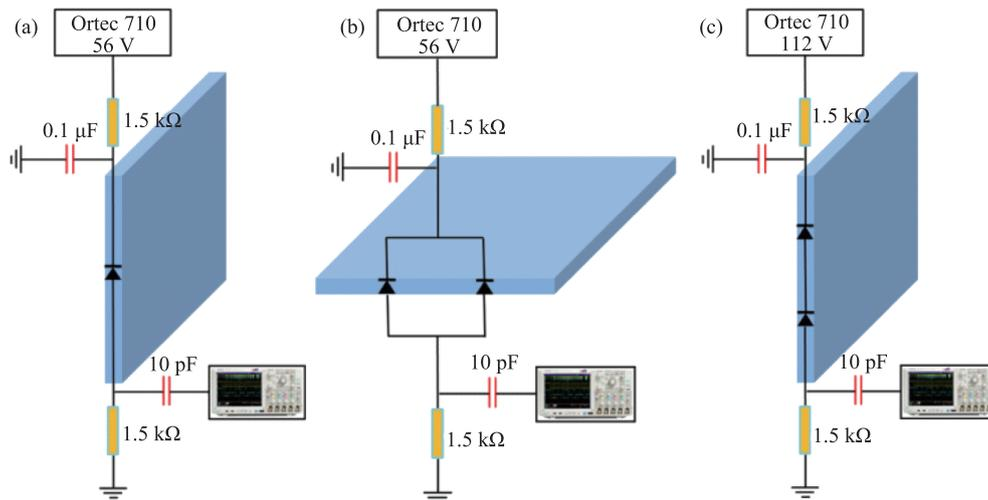
Fig. 1 (color online) Schematics of the setups for measuring the signals with different SiPM connections. (a) A single SiPM. (b) Two SiPMs connected in parallel. (c) Two SiPMs connected in series.
