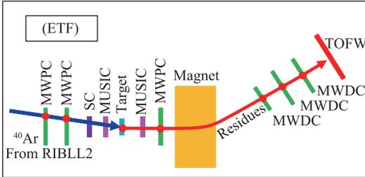
Fig. 1 (color online) Layout of the External target Facility.
