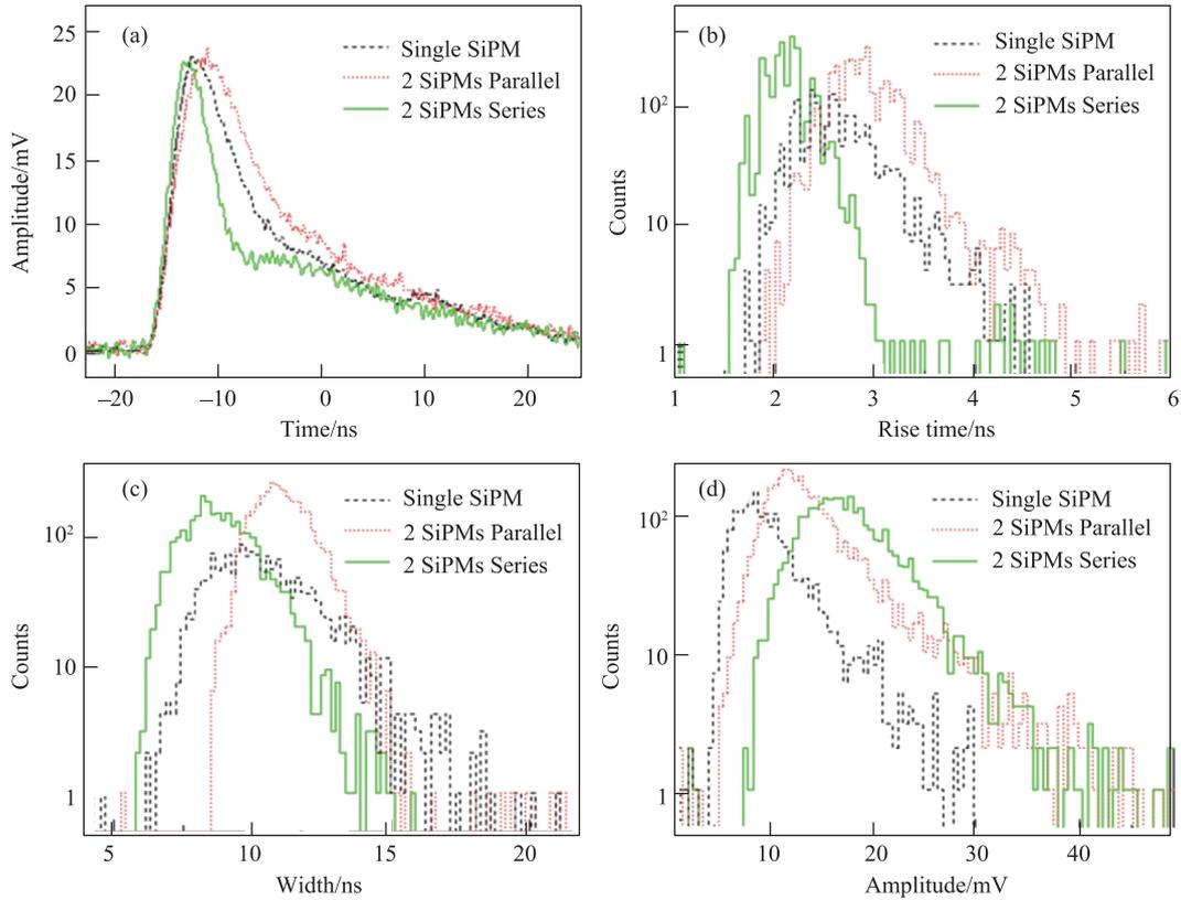
Fig. 2 (color online) Test results with cosmic rays. The signal shapes, the rise time distributions, the width distributions, and the amplitude distributions with different SiPM connections are shown in (a), (b), (c), and (d), respectively.
