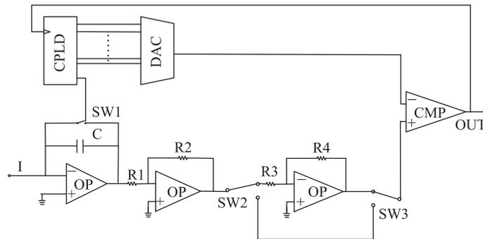
Fig. 1 Principle diagram of the current to frequency converter.
