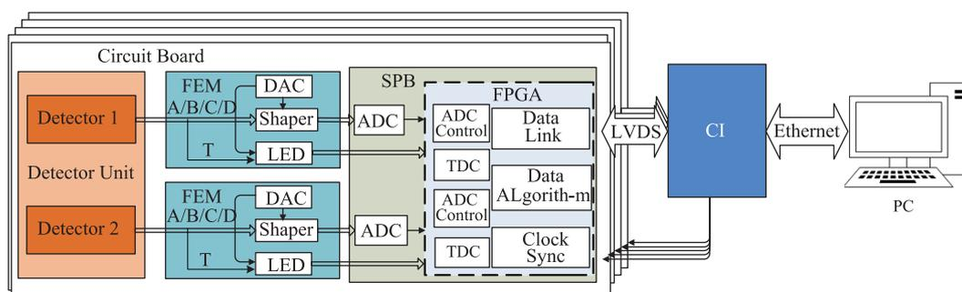
Fig. 1 (color online) The TOF-PET system architecture.
