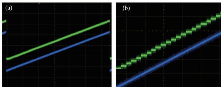
Fig. 2 (color online) output waveform of the circuit. (a) the output waveform of a single operating cycle; (b) a partial waveform of (a).
