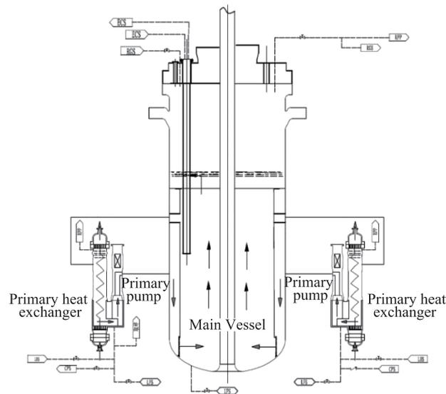
Fig. 2 Scheme of main coolant system.
