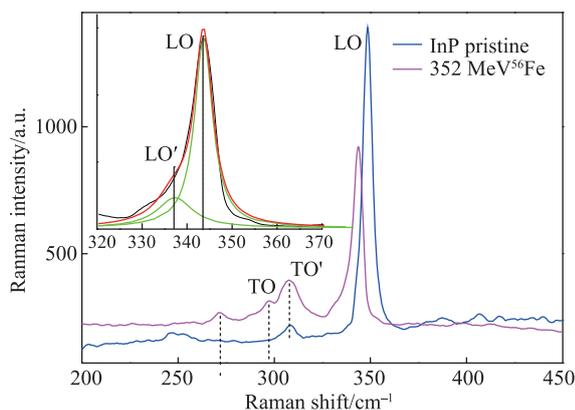
Fig. 1 (color online) Raman spectra of InP before and after irradiation.
