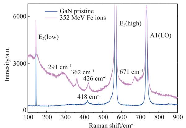
Fig. 2 (color online) Raman spectra of GaN before and after irradiation.
