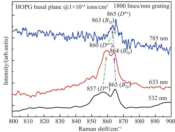
Fig. 4 (color online) The Raman spectra of the basal plane of the irradiated graphite with 40.5 MeV Sn ions using three different excitations.
