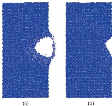
Fig. 1 (color online) Snapshots of the crater formation process in 13.8 nm gold nanowire induced by 20 keV PKA irradiation at the surface. (a) at 10.5 ps and (b) at 80.0 ps.
