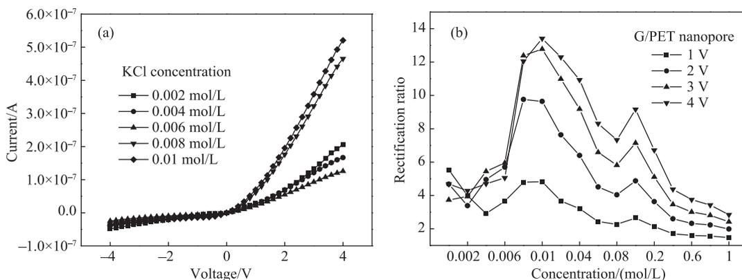
Fig. 1 Rectification of G/PET nanopore. (a) current-voltage curves of G/PET nanopore with an applied voltage ranging from -4 V to 4 V in KCl electrolyte with different concentrations, (b) The ion rectification ratio as a function of KCl electrolyte concentration at different applied voltages.
