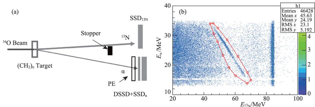
Fig. 1 (color online) (a) The experimental setup. (b) The energy correlation of  $\alpha$  and  $^{13}\text{N}$ .
