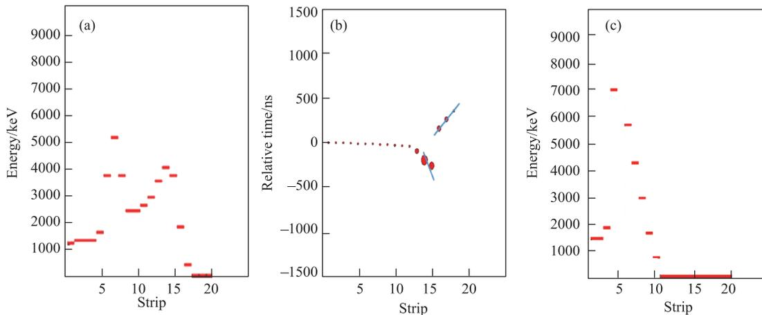
Fig. 2 (color online) (a) A scattering event with two peaks. (b) The relative time of heavy ions on different strips. (c) A confusing event with both fusion and scattering characteristics.
