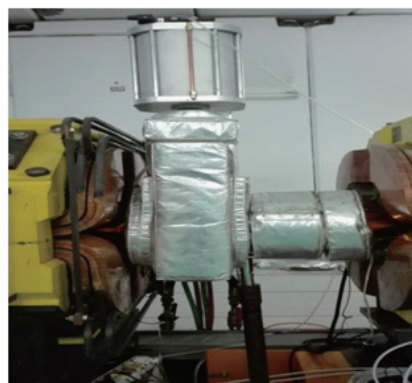
Fig. 2 (color online) Installation of a all-metal CF200 valve.
