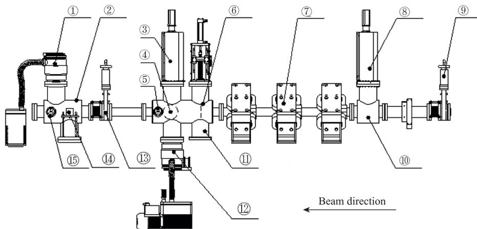
1. Molecular pump A; 2. Test chamber A; 3. Fluorescent target A; 4. Faraday Cup; 5. Vacuum gauge A; 6. Copper slit; 7. Quadrupole magnets; 8. Fluorescent target B; 9. Vacuum valve A; 10. Vacuum chamber B; 11. vacuum chamber C; 12. Molecular pump B; 13. Vacuum valve B; 14. Oxygen-Free Copper; 15. Vacuum gauge B.
