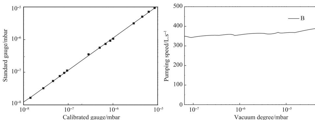
Fig. 3 The results of the gauge calibration and pumping speed measurement.
