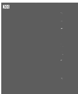
Fig. 2 Pixel image of water droplets with 45 ° between laser and camera.
