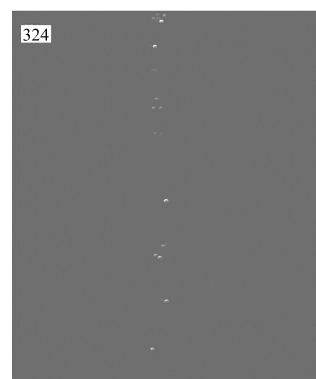
Fig. 3 Pixel image of droplets with 135 ° between laser and camera.
