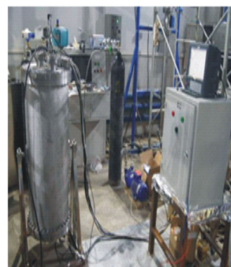
Fig. 6 (color online) The facility for static granular heat transfer experiments.
