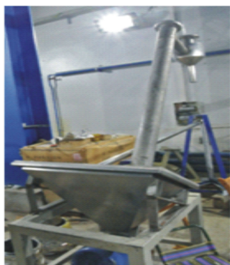
Fig. 4 (color online) The oblique spiral hoist with an inclination angle of 60°.
