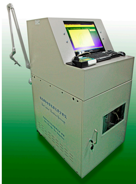
Fig. 1 (color online) Picture of the moveable LIBS instrument.
