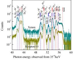
Fig. 1 — (color online) Decay X-ray spectrum of the scattered  $Xe^{53+*}$  and  $Xe^{52+*}$  in 94 MeV/u  $Xe^{54+}$  collision with Kr and Xe atoms, observed from 35°. The counts of the Kr target are divided by 10 to shift the plot.
