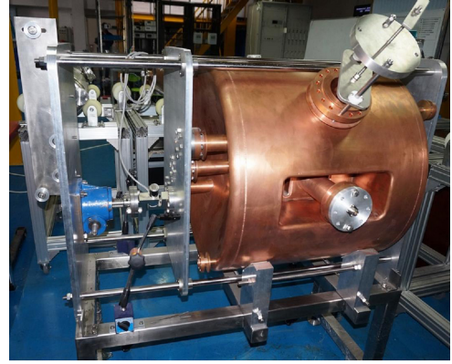
Fig. 3 (color online) Overall setup for the bead-pull and tuning test device.
