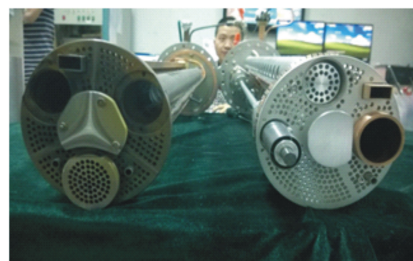
Fig. 2 (color online) The old and new injection components of SECRAL.
