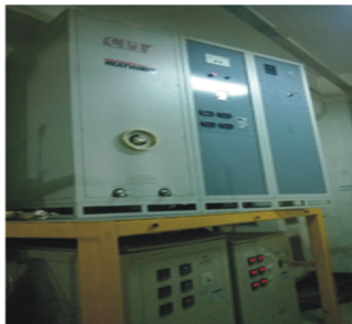
Fig. 5 (color online) The 28 GHz microwave Generator.
