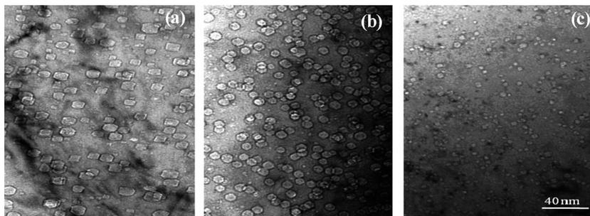
Fig. 2 Microstructure of cavities in Japan T91 steel at different irradiation conditions. (a) 31 dpa, RT; (b) 28 dpa, 450 °C; (c) 31 dpa, 550 °C.
