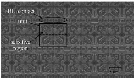
Fig. 1 SEM picture of the layout of IDT71256 SRAM cells. Every unit contains four memory cells. SEU sensitive region of the 4-transistor, polysilicon resistor load SRAM cell is the drain of the off-transistor.
