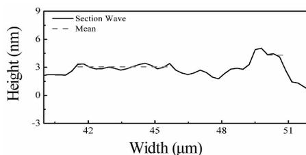
Fig. 2 The section wave correspond to the straight line on AFM image.
