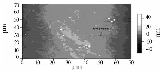
Fig. 1 AFM image of graphene sheets with different thickness.
