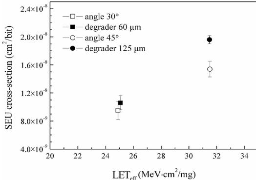
Fig. 1 The SEU cross section as a function of  $LET_{\text{eff}}$ . The error bars represent the standard deviation.
