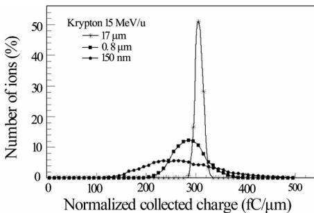
Fig. 1 Simulated number of ions as a function of the deposited charge, normalized to the silicon film thickness, induced by the energy the ion deposited in the sensitive volume, for 25 MeV/u krypton ions in devices with different silicon film thicknesses.
