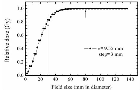
Fig. 2 The dependence of central dose on calibration field size.
