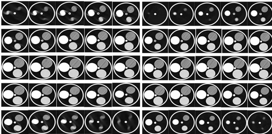
Fig.1 Axial slices of the moving phantom. Window level 1200 centred at  $-600$ . 1.5 mm slice, 1.5 mm reconstruction increment, 50% exhalation (left) and 0% exhalation (right).
