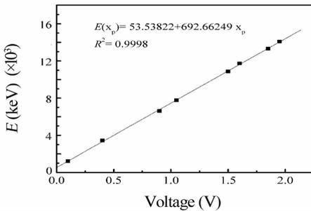
Fig. 1 Linear fitting between the  $\gamma$  ray energy and the threshold voltage.
