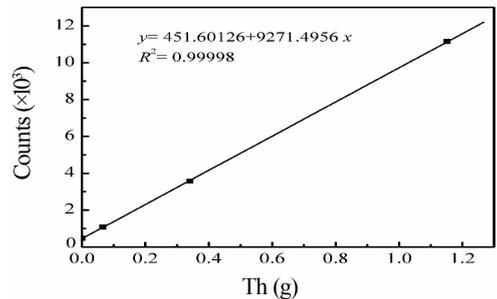
Fig. 3 The count of standard thorium samples vs the weight of  $^{232}\text{Th}$  content.
