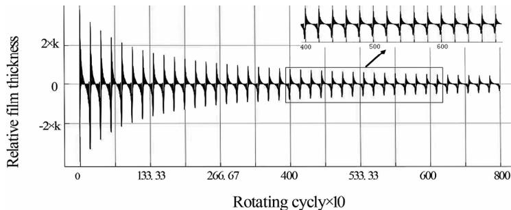
Fig. 1 Simulation on the relationship between the thickness-uniformity and the wafer rotating cycle. The target horizontally moving period is fixed to be 2 min.
