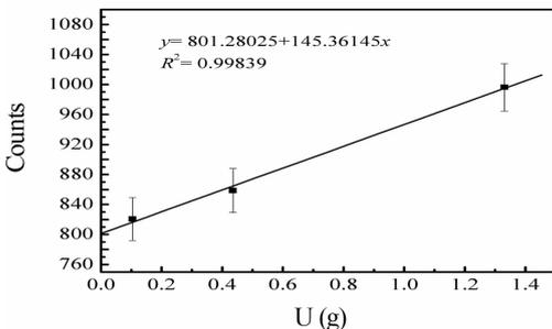
Fig. 2 The count of standard uranium samples vs the weight of  $^{238}\text{U}$  content.
