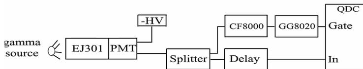
Fig. 1 Experimental setup and electronics setup of electron responses measurement of gamma source.
