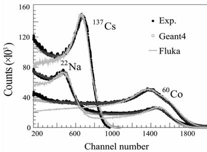
Fig. 2 Comparison of experimental light output with simulation results.
