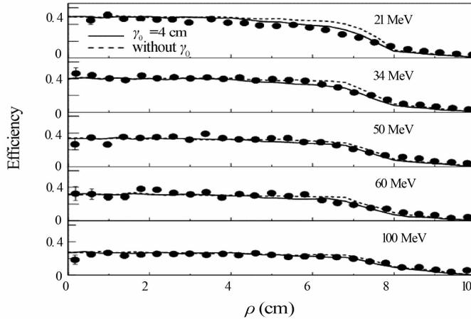
Fig. 2 Neutron efficiencies as a function of radius.  $\bullet$  the experimental data,  $-$  and  $---$  with  $r_0$  and without  $r_0$  correction.
