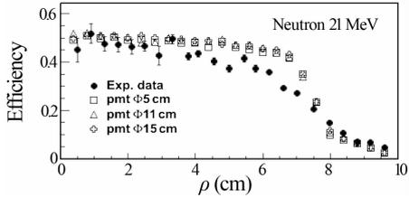
Fig. 1 Comparison between neutron efficiencies at 21 MeV vs radius of scintillator with different PMT diameters and experimental data.
