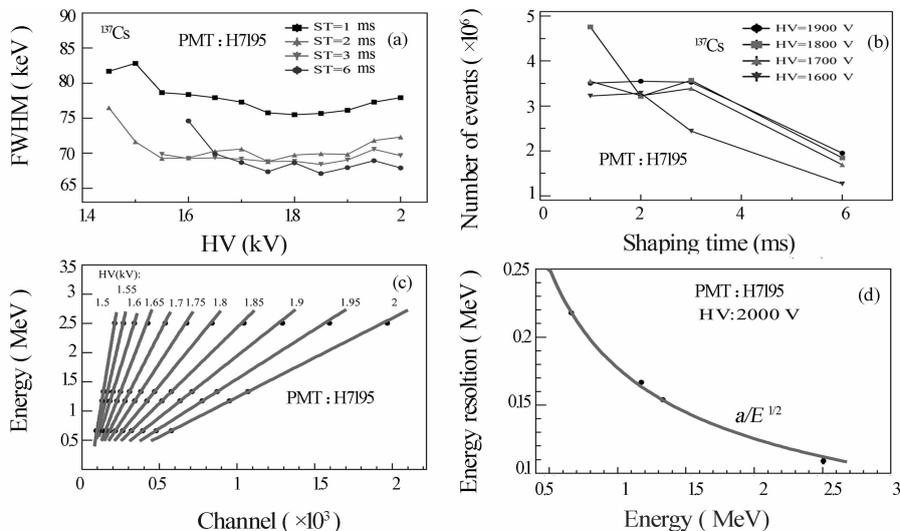
Fig. 1 (a) Energy resolution as a function of bias voltage. (b) Data acquisition count rate as a function of the shaping time. (c) Energy calibration curve in different bias voltage. (d) Energy resolution as a function of source energy.
