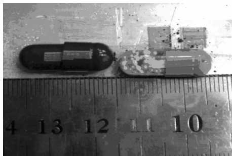
Fig. 1 The capsule after laser ablated.
