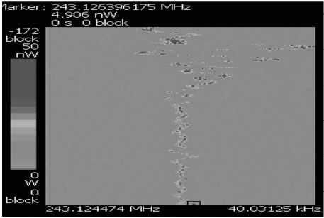
Fig. 2 Beam spectrum of resonant Schottky pickup in CSRe.
