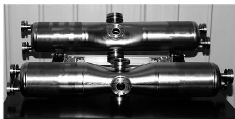
Fig. 3 The two fabricated superconducting HWRs.
