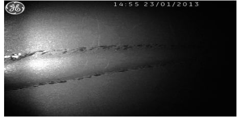
Fig. 6 Internal conductor after second time polishing.
