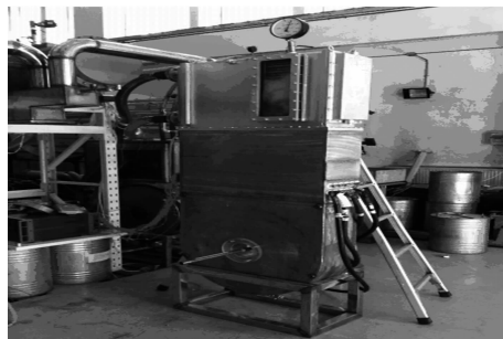
Fig. 2 Prototyped mirror solenoid magnet for LECR4 ion source.
