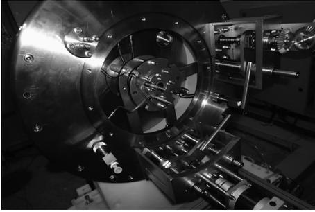
Fig. 5 The three-electrode extraction system.
