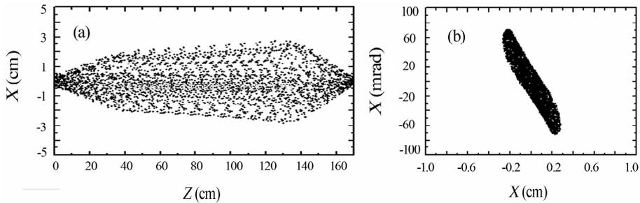
Fig. 2 (a) BEAMPATH simulated beam trajectories along the length of C-ADS LEPT; (b) Simulated phase space distributions.
