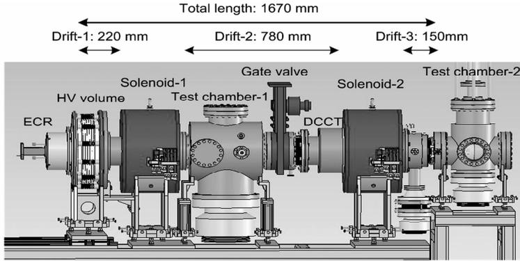
Fig. 1 Layout of the LEPT for C-ADS where the Test Chamber-2 takes the place of the RFQ for early development.
