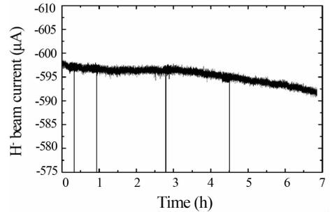
Fig. 6 Beam stability within 7 h.
