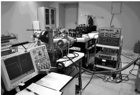
Fig. 1 The beam test platform of DWA as a diode.
