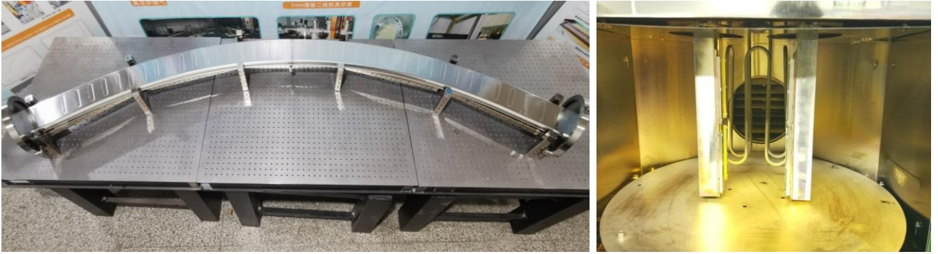
Fig. 5 Prototype of ultra-thin walled ultra-high vacuum chamber with ceramic lining (left) and the device for magnetron sputtering gold-plated film on ceramic ring (right)
