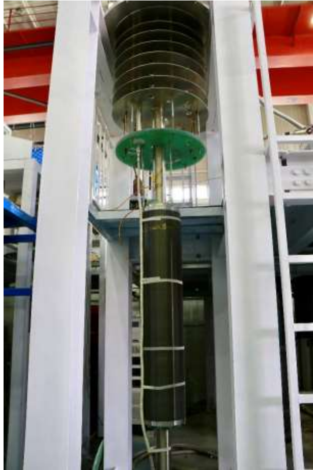
Figure 2.8 Prototype of the quadrupole and sextupole (Q&S) combination with half-aperture
