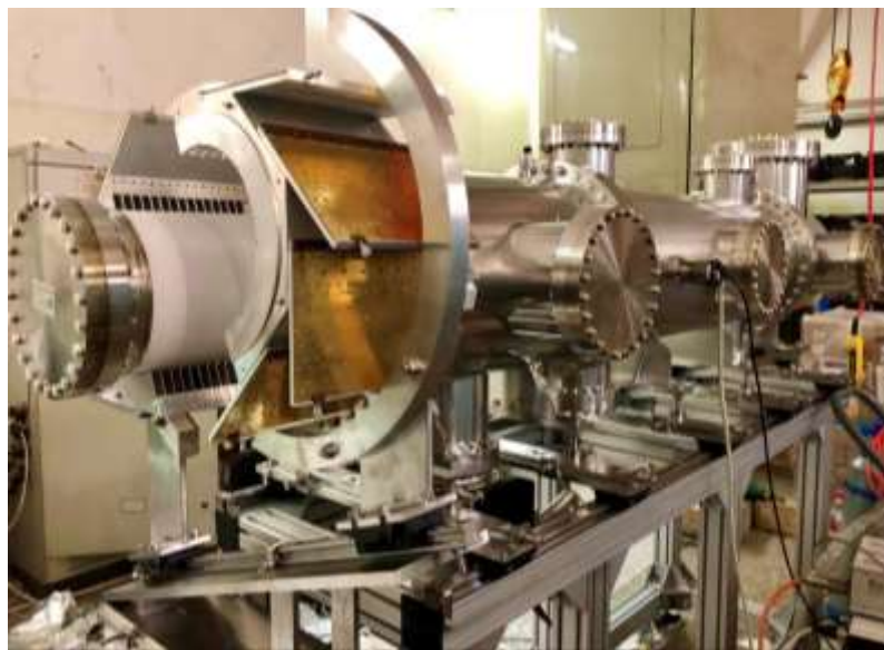
Figure 2.12 Pick-up for SRing stochastic cooling system
