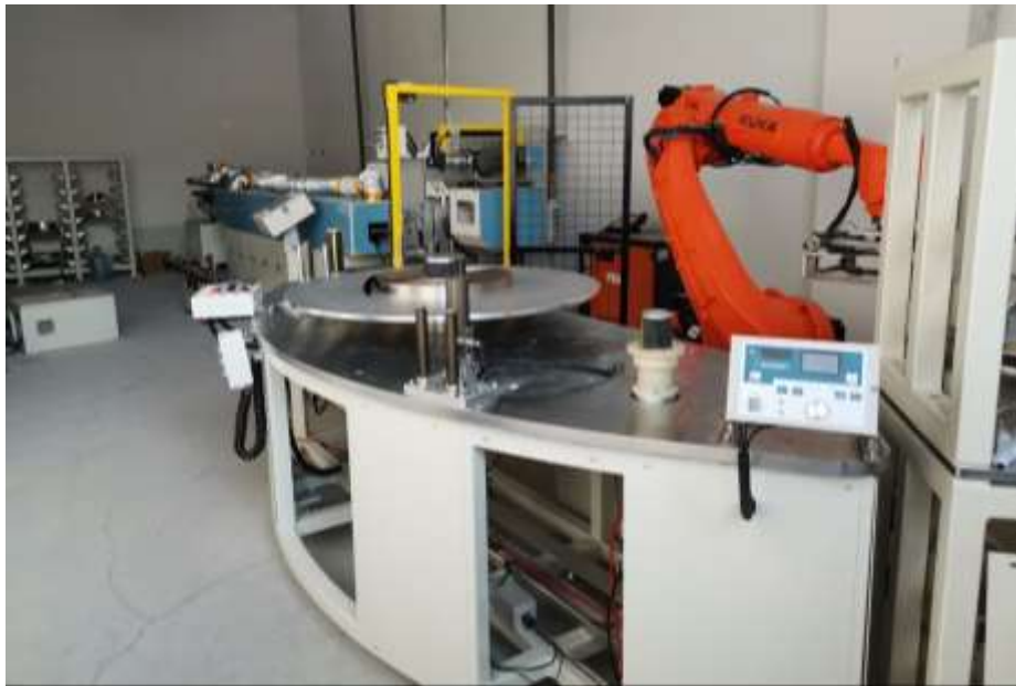
Figure 2.5 Equal tension horizontal winding system for core manufacture
