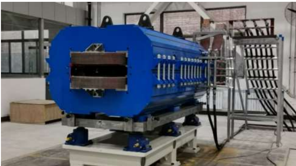
Figure 2.7 Full-size prototype of the fast ramping dipole magnet for BRing
