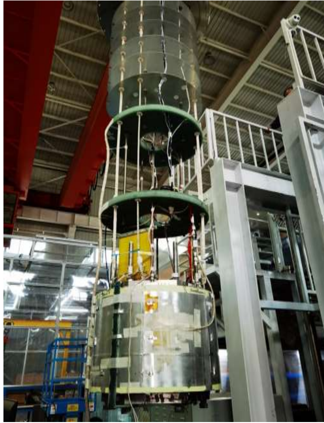
Figure 2.1 Prototype of the first Nb 3 Sn superconducting Electron Cyclotron Resonance (ECR) ion source magnet cold mass
