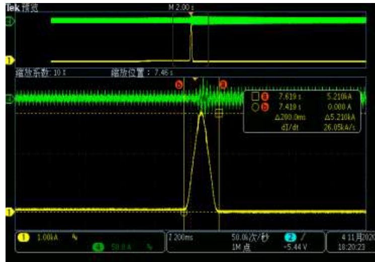
Figure 2.3 Output current of 5200A in pulse mode by the prototype
