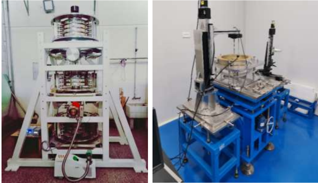
Figure 2.11 Electron cooler test bench (left) and magnetic field measurement platform for coils (right)
