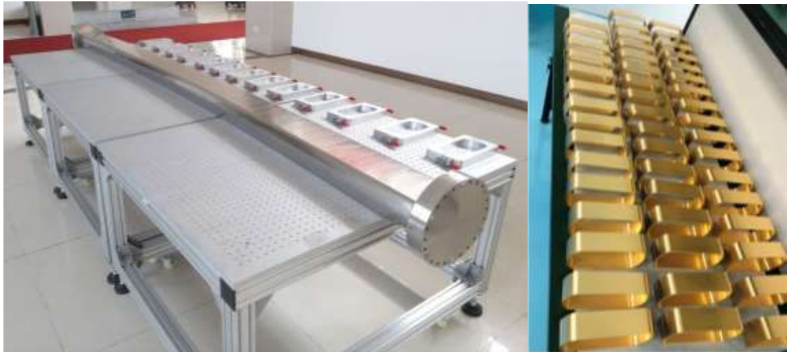
Figure2.6 Prototype of the ultra-thin-wall XHV chamber (left) and Au/Ti/Cu/Ti multilayer coating ceramic ring (right)
