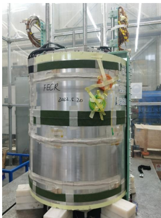
Figure 2.1 Full-sized Nb 3 Sn ECR ion source cold mass
