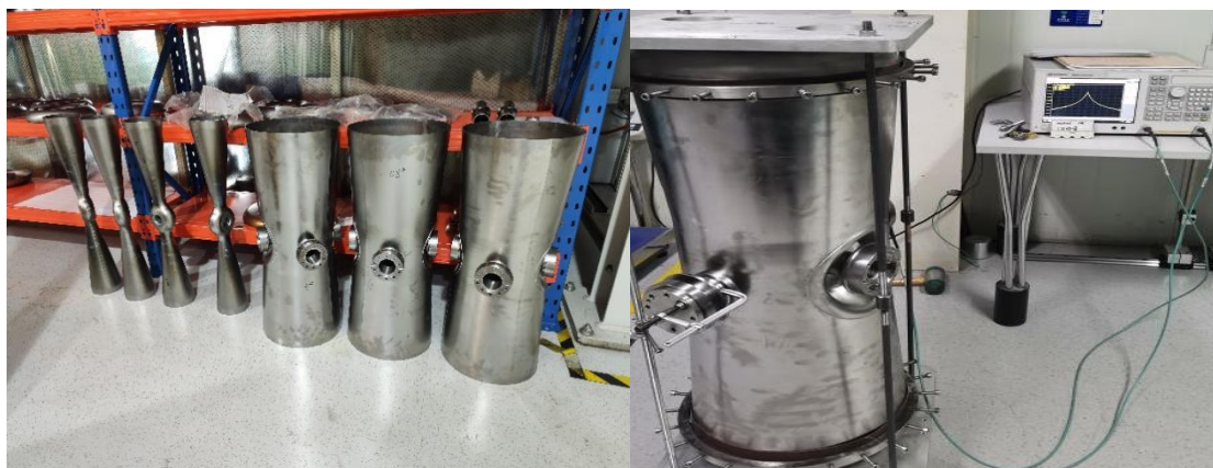
Figure 2.10 Superconducting RF cavities of iLinac
