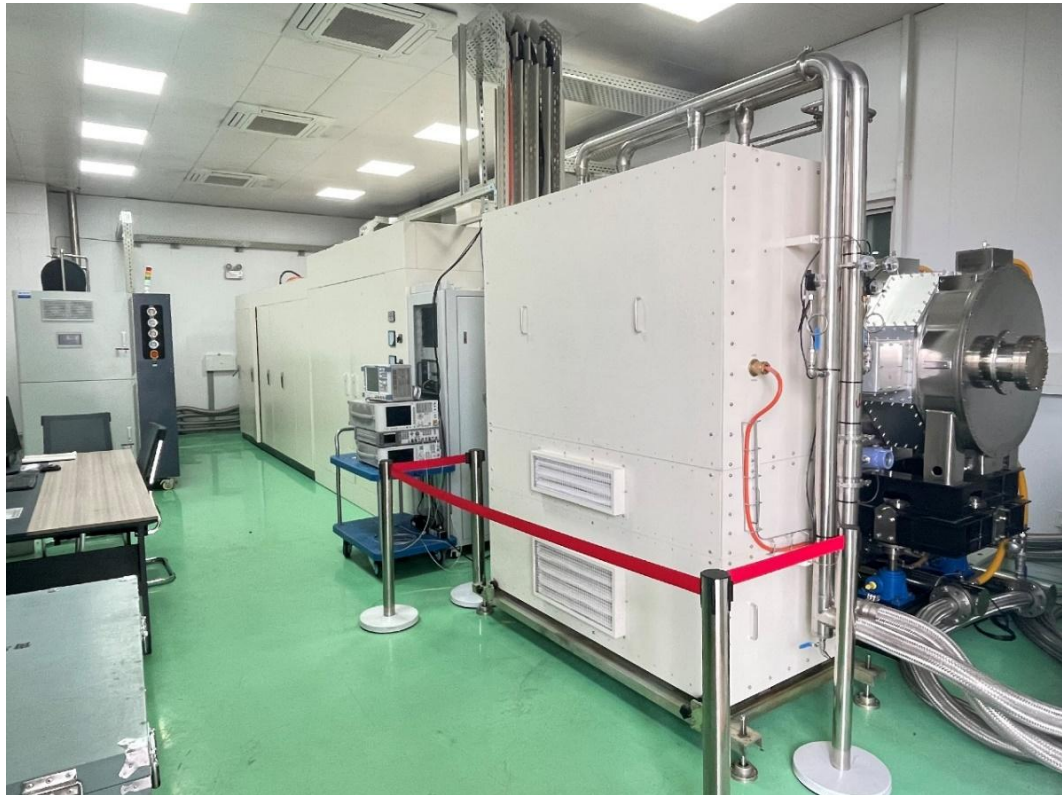
Figure 2.6 The high-performance MA-load RF system
