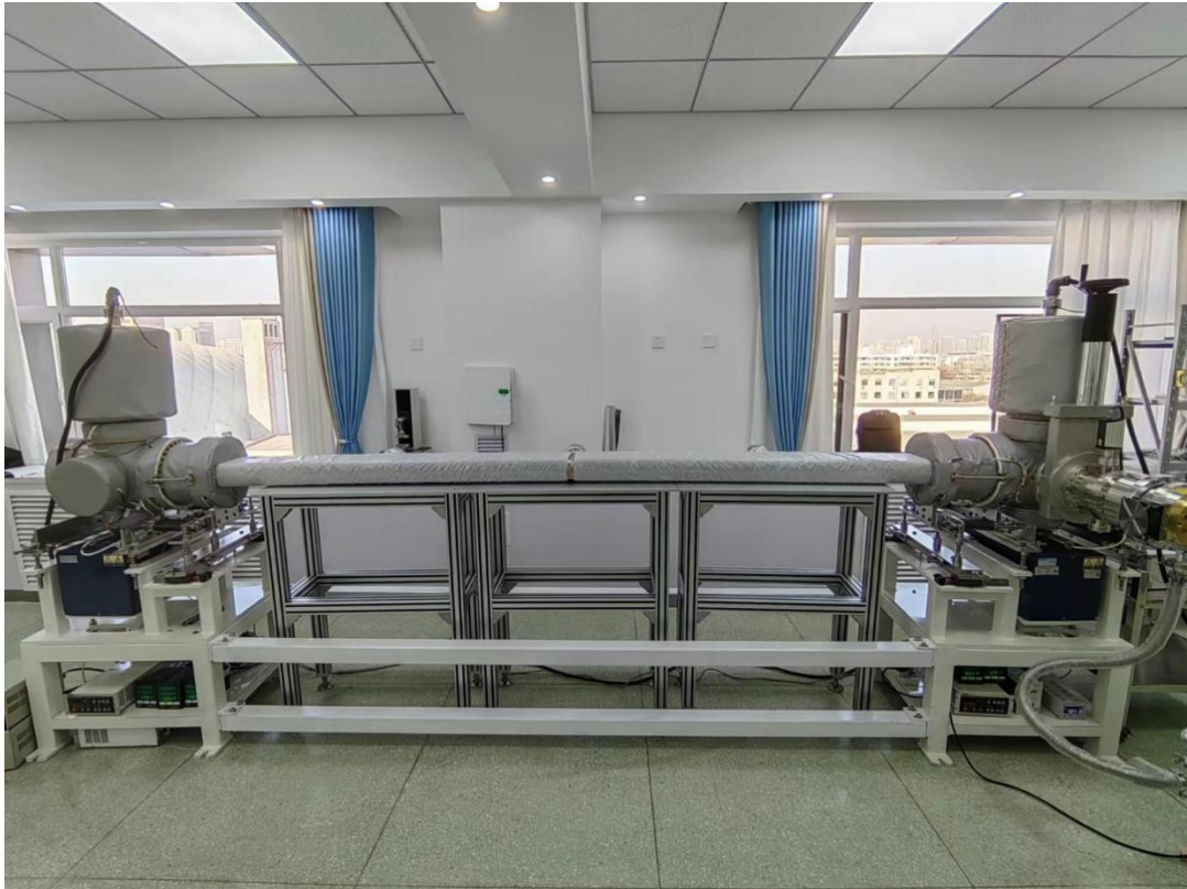
Figure 2.5 The first set of the Titanium alloy lined high-vacuum chamber with ultra-thin wall
