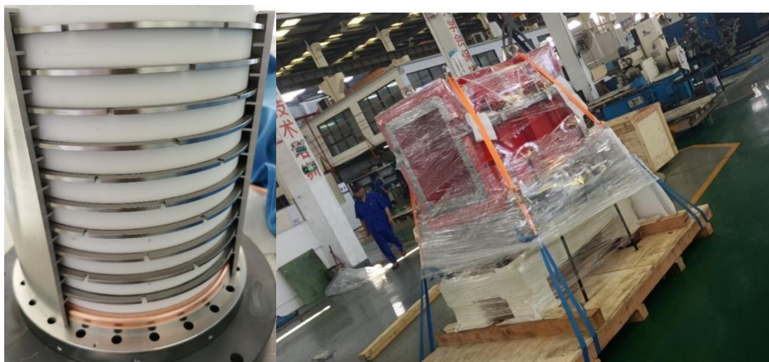
Figure 2.15 Acceleration tube and magnetic yoke of the electron cooler in SRing
