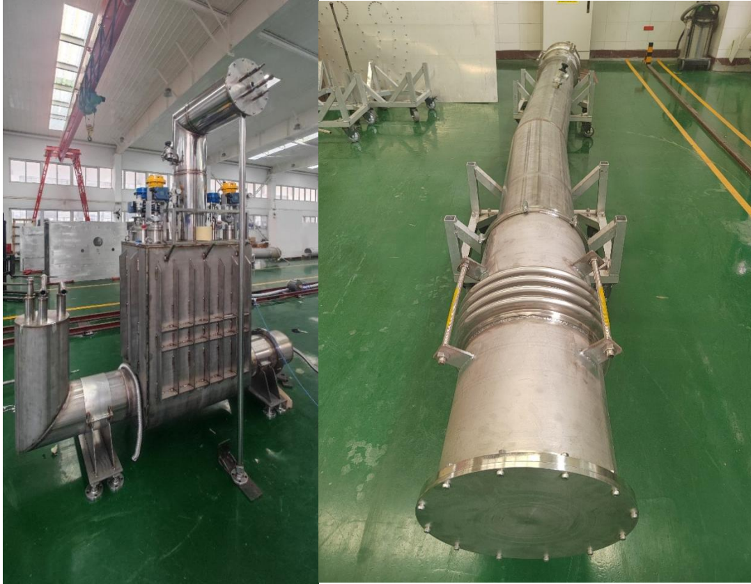
Figure 2.23 The valve box and the pipeline of HFRS sectional mockup
