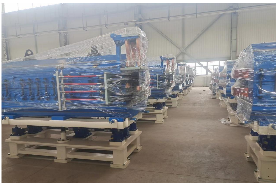
Figure 2.12 Dipole magnets of BRing
