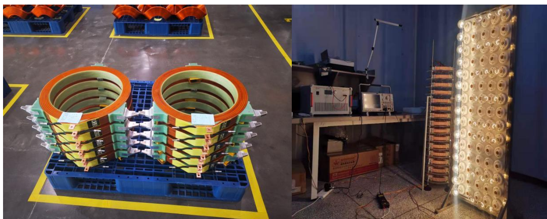
Figure 2.20 The high-precision solenoid coil (left) and the isolation transformer (right) in the electron cooling system
