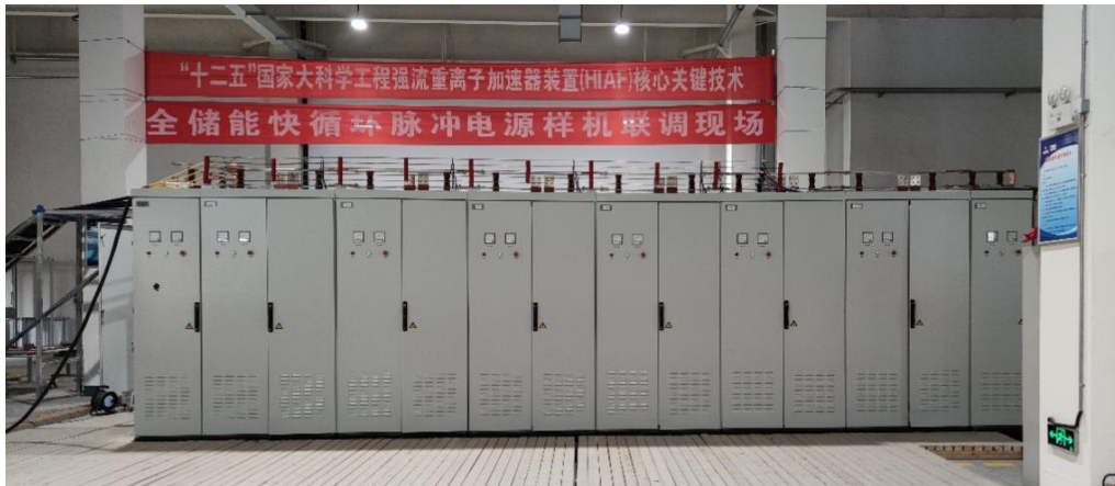
Figure 2.4 Prototype of the full-energy-storage fast-cycling pulse power supply
