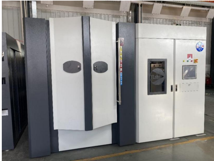
Figure 2.8 Magnetron sputter coating machine for ceramic ring
