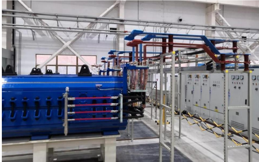
Figure 2.7 United test platform for the dipole ramping
