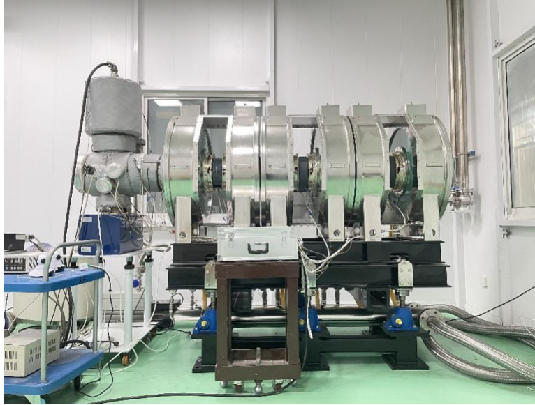
Figure 2.3 MA loaded RF cavity prototype under test (vacuum: 5.5 \times 10^{-12} mbar)
