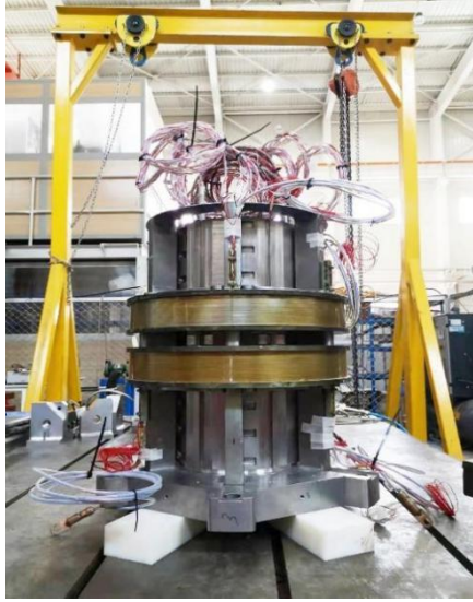
Figure 2.1 Nb 3 Sn ECR ion source cold mass
