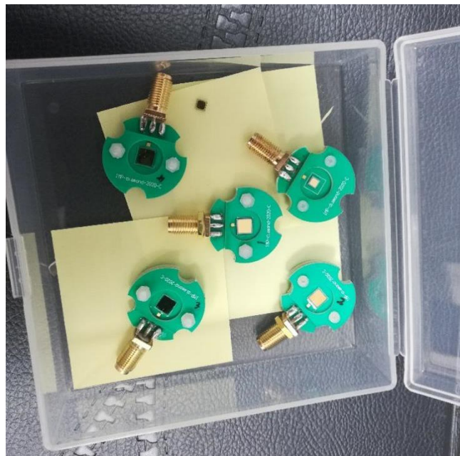
Figure 2.22 The diamond time-of-flight detector prototype
