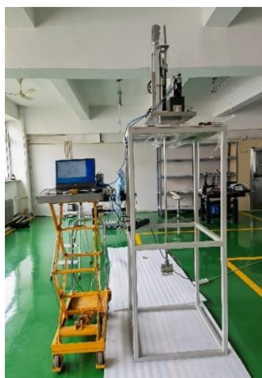
Figure 2.24 The prototype of HFRS radiation-resistant fluorescent target
