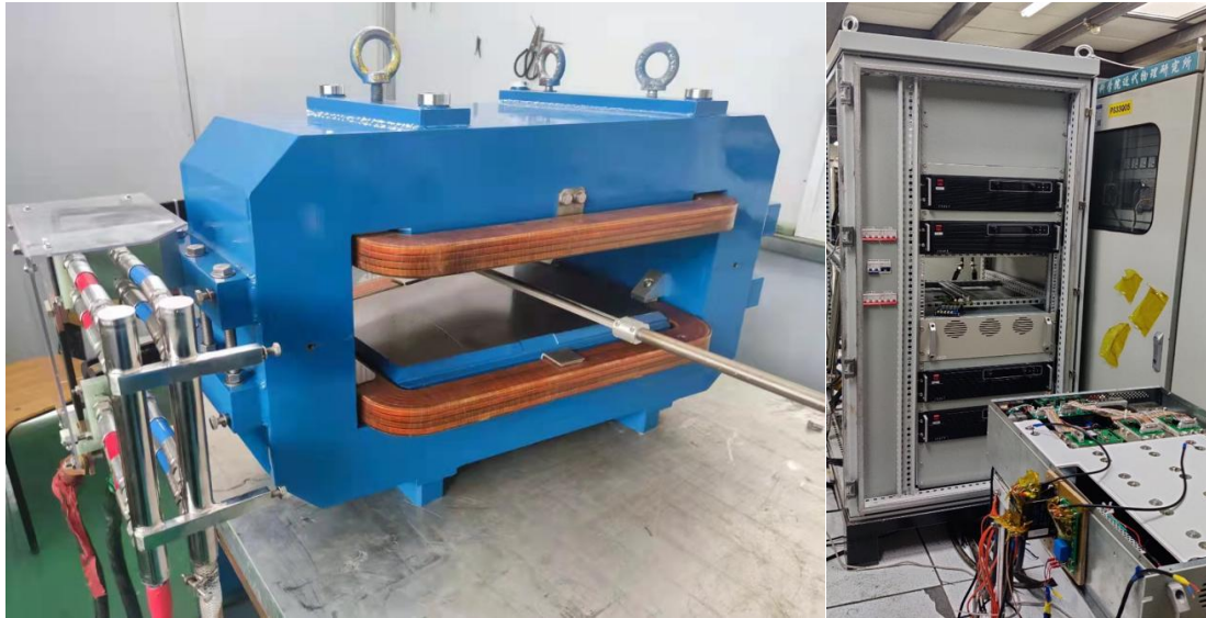
Figure 2.12 The 45 degree fast-chopper magnet (left) and its power supply (right) in front-end system
