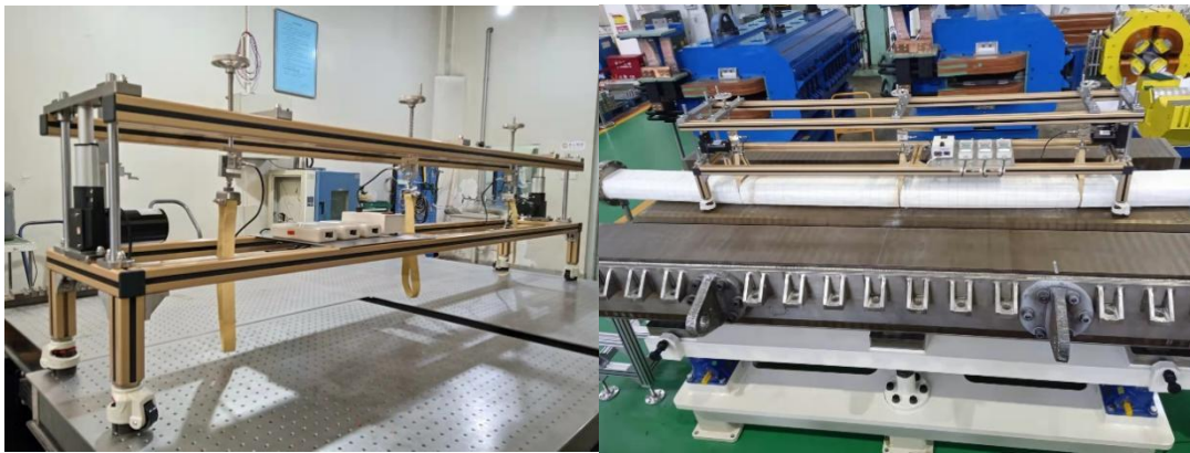
Figure 2.9 Combined test of the lifting support stand for ceramic-lined thin-wall vacuum chamber with the dipole magnet
