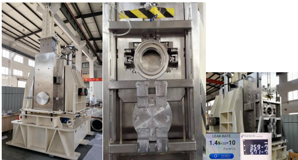
Figure 2.23 The prototype processing and the joint test between HFRS primary target chamber and pillow seal
