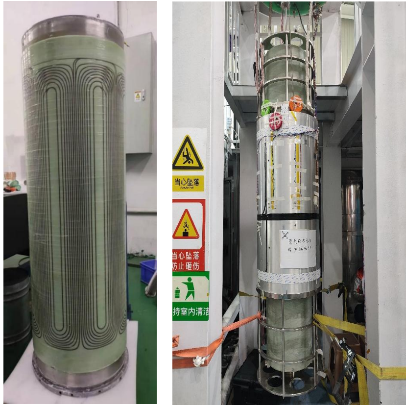
Figure 2.10 Full-aperture superconducting multipole combined prototype magnet and the low temperature test components
